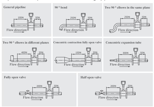
Vortex flowmeter has certain requirements for the upstream and downstream straight pipe sections of the installation point, otherwise it will affect the flow field of the medium in the pipeline and affect the measurement accuracy of the instrument.
